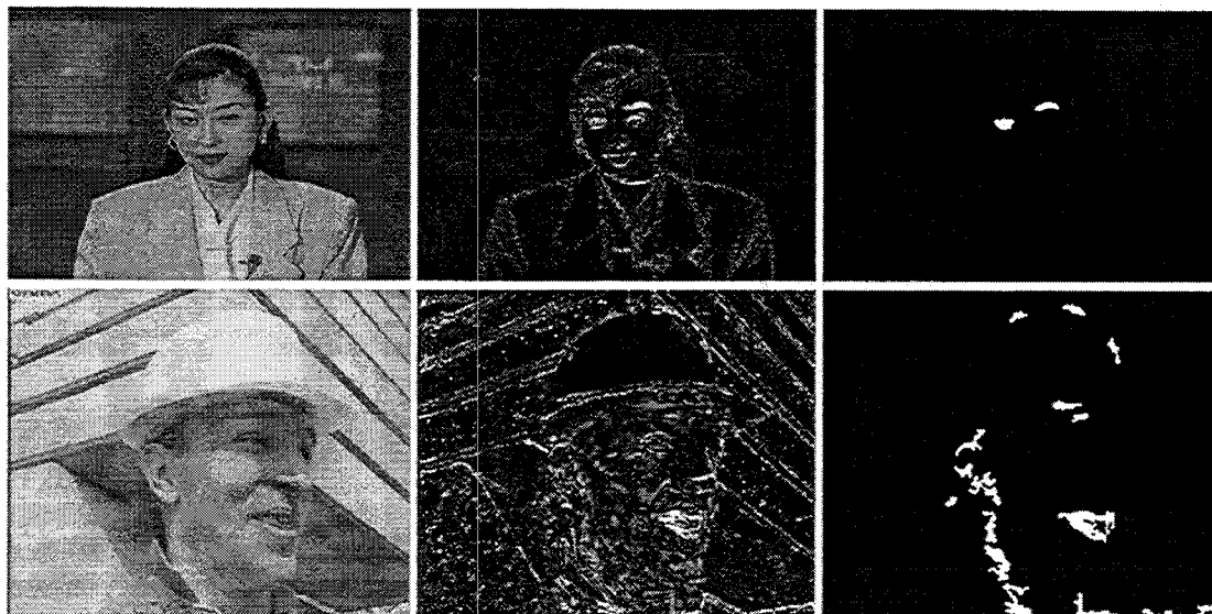
Figure 1. Original frame, DFD (absolute value) and update signals created by the morphological segmentation algorithm (black denotes inactive and white active areas). Top: 'Akiyo', bottom: 'Foreman'.
