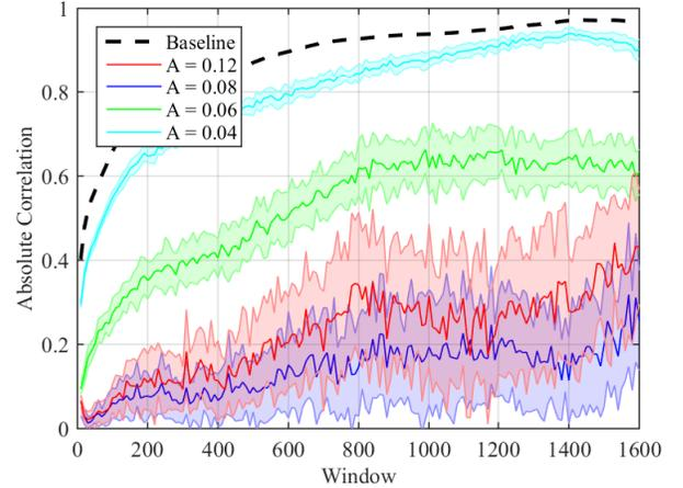
Fig. 6. The effectiveness of the proposed privacy enhancement scheme for various thresholds ( $A$ ). The solid lines correspond to the mean and the shade corresponds to one standard deviation over 20 runs ( $L = 3$ ).
