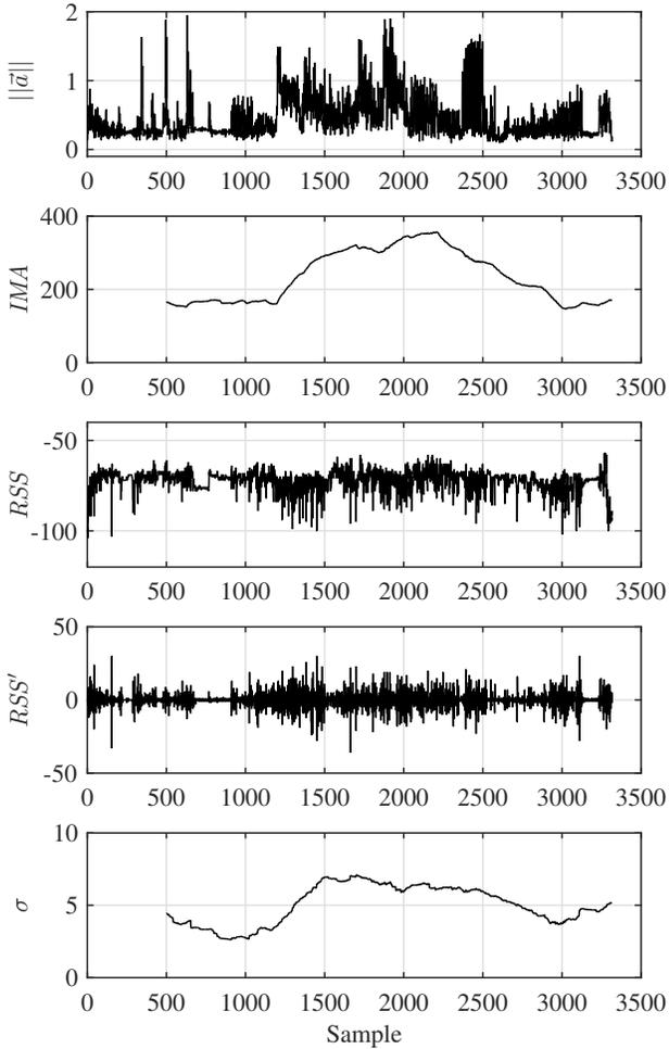
Fig. 2. Experimental results on the first session yield very strong correlation ( $c = 0.87$ ) between the physical activity levels ( $IMA$ ) and the standard deviation of the derivative of the  $RSS$  ( $w = 500$ ). The magnitude of the acceleration,  $\|\vec{a}\|$ , is in g-units. The received signal strength,  $RSS$ , is in dBm. Its derivative,  $RSS'$ , is in dBm per sampling period.
