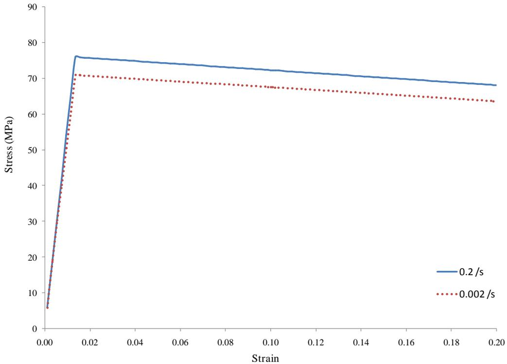
Fig. 3. Effect of applied strain rate on response of single element model
